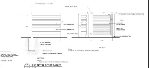
4" BALL CAP-4"x4"x1/4" BASE PLATE — TO CONTINUOUS CONC.
