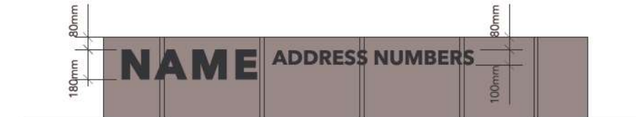
3 ADDRESS SIGN DETAIL Scale: 1:10
