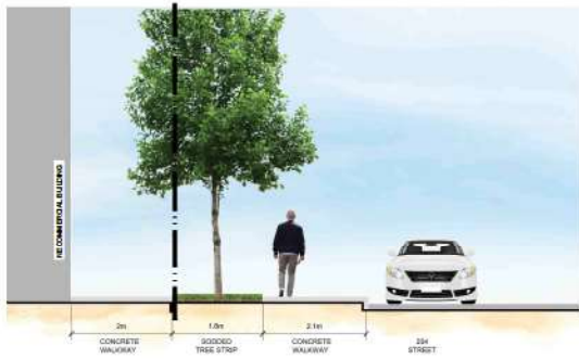
S2 SECTION THROUGH EAST PEDESTRIAN CORRIDOR 1:50
