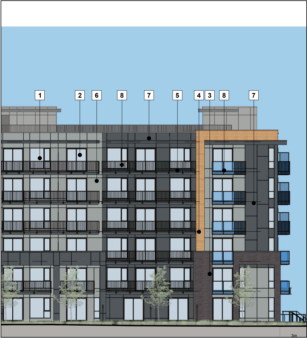
* NOTE: All fiber cement panels trims/recess, reveals, reglets, etc. must be colored matching to the panels they are attached to.
