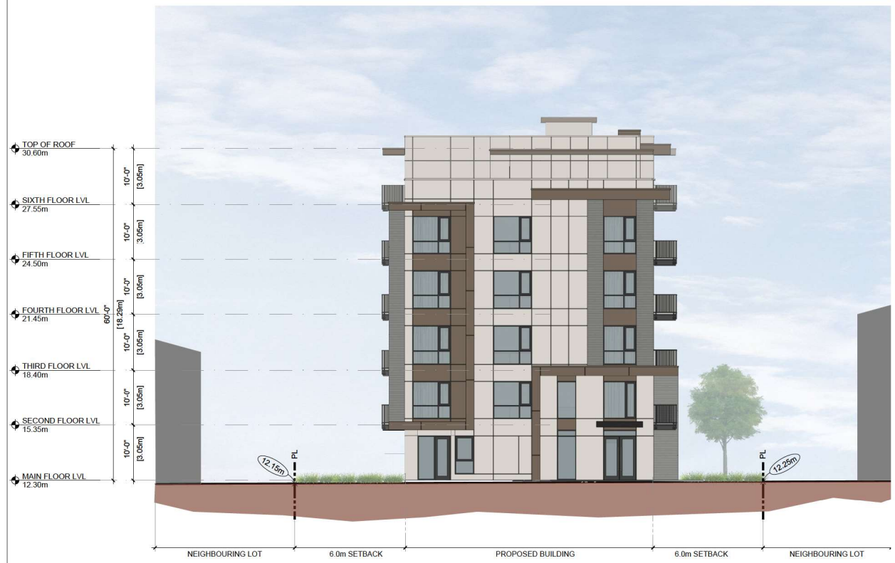
1 NORTH ELEVATION (ALONG 56 AVENUE) Scale: 1/16" = 1'0"
