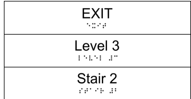
3.4.5.2. & 3.4.6.19. Examples of Exit, Stair & Floor Sign Info
