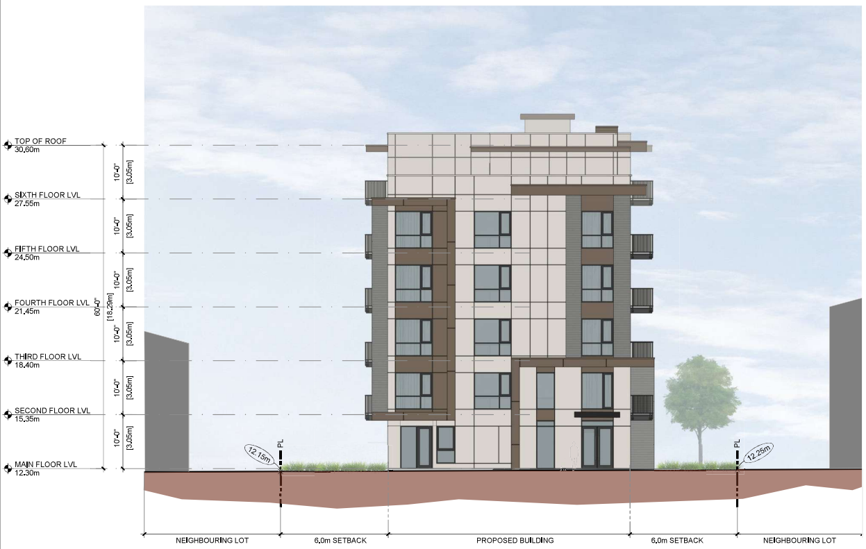
1 NORTH ELEVATION (ALONG 56 AVENUE) Scale: 1/16" = 1'0"
